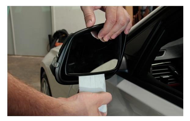
3. You'll see the wires for the mirror lens/heating element. They do not need to be unclipped if you rest it on the window sill.
