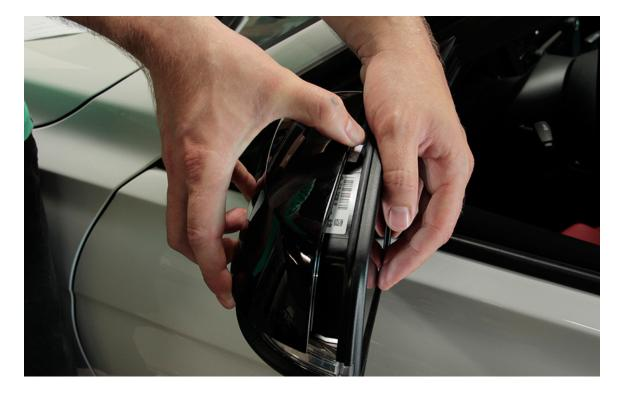
1. Grab and pull the OEM cap off starting from the top edge, then pull straight out.
