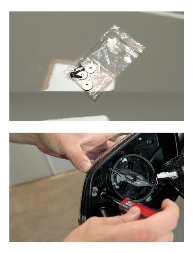
8. Install hardware, and clip mirror back in, so that it's orientated with the plastic receivers.
