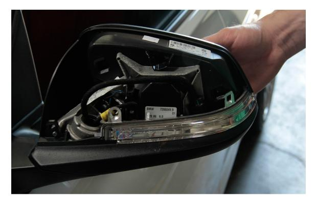
2. Tilt the mirror lens up as much as possible, then using a plastic panel tool or similar pull the lens outward at a slight upward motion.
