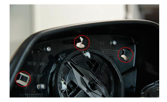
4. Locate the 3 tabs that are located where the OEM cap clips in.
